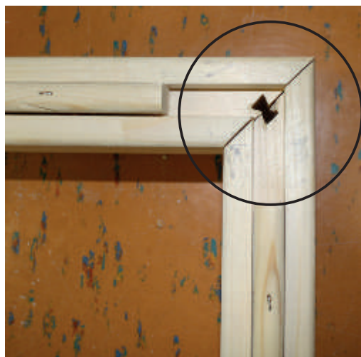
Fig. 2: Connect the floor frame elements
