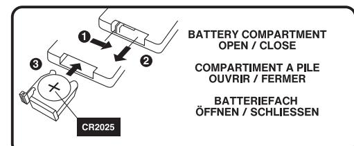
> When the lamp no longer responds to the signal from the remote control, replace the original battery with a new 3V CR2025 lithium battery.
